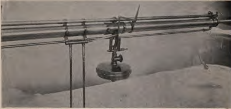
Fig. 52.—Gyroscope, used for the control of the fore and aft horizontal rudders, thus keeping the machine on an even keel while in the air.
